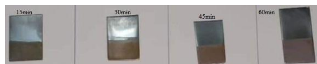
Fig.3 \text{Cu}_2\text{O} thin films deposited at different time values.
