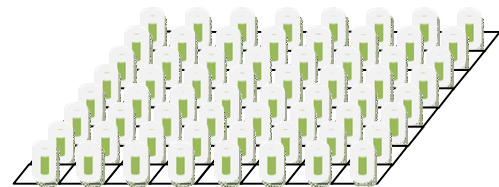
Fig.1 A periodic structure of carbon nanotube in Thz application
