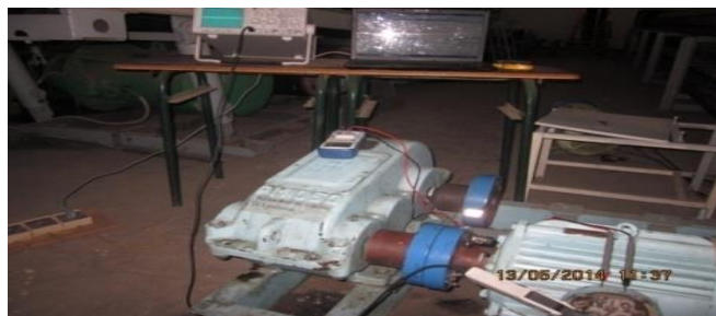
Fig. 4 Test bench of the electromechanical drive system engine – reducer
