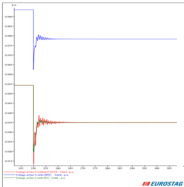
Fig. 12. Voltage magnitude at bus 9 without and with FACTS.
