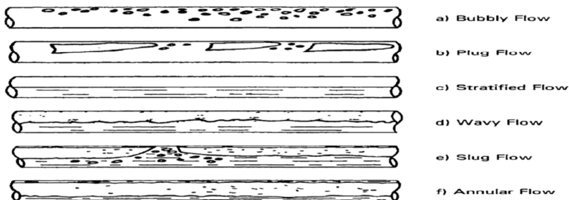
Figure 1. Some flow patterns in horizontal pipe.
