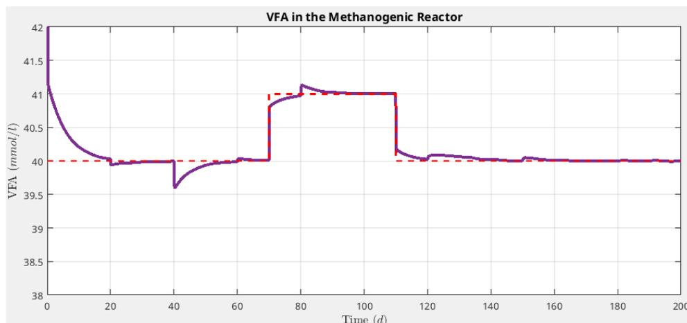
Fig. 5 Dynamical behaviour of VFA in the methanogenic bioreactor (continuous line) with to the set-point (dashed line).
