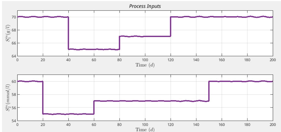
Fig. 2 Process inputs: COD ( $S_1^{in}$ ) and VFA ( $S_2^{in}$ ).
