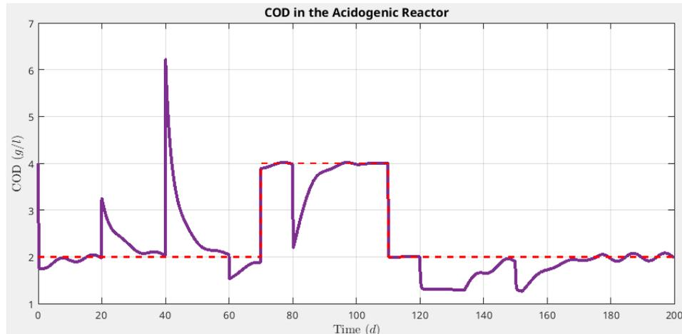
Fig. 4 Dynamical behaviour of COD in the acidogenic bioreactor (continuous line) with to the set-point (dashed line).
