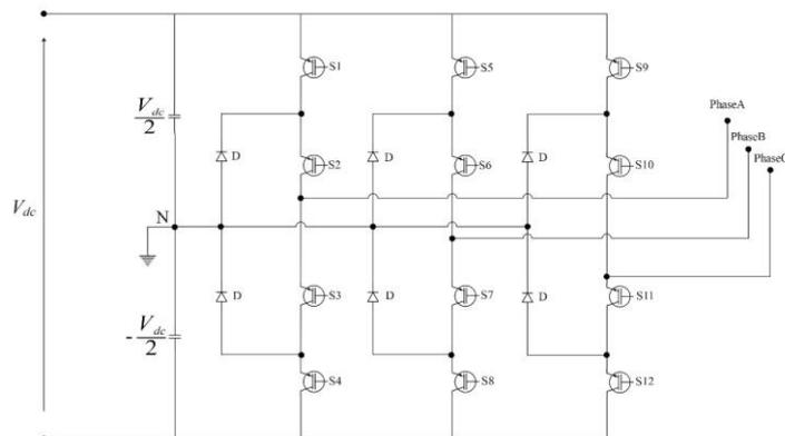
Figure 9 three phases NPC inverter 3 level
