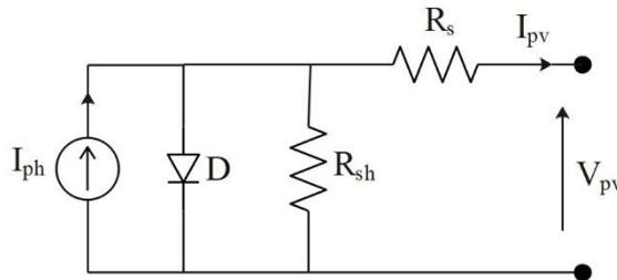
Figure 7 Equivalent Circuit Model of a Photovoltaic Cell
