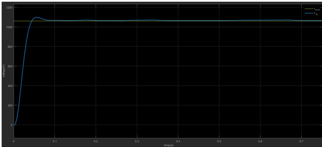
Figure 21 control of input inverter voltage  $V_{dc}$
