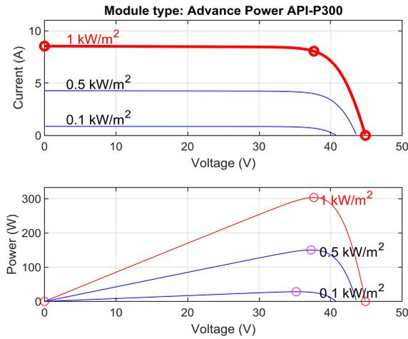
Figure 3 I-V and P-V Characteristics of a Photovoltaic Module under Different Irradiance Levels
