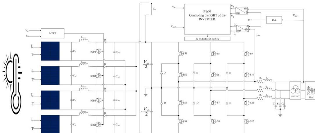
Figure 1 Schematic of a Grid-Connected Photovoltaic System with MPPT, Boost Converters, and PWM-Controlled Inverter for Optimal Power Conversion
