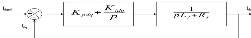
Figure 12 Current Regulation Using PI Control in dq Frame
