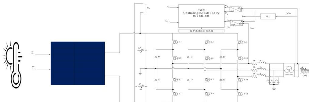
Figure 2 Schematic of a Grid-Connected Photovoltaic System PWM-Controlled NPC Inverter, and Without Boost Converter
