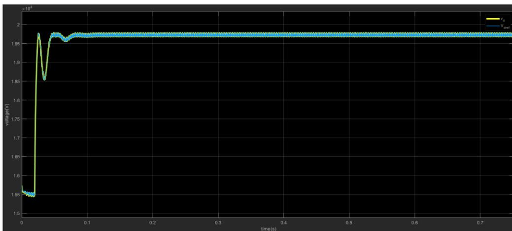
Figure 22 control of the output voltage in frame d  $V_d$  and  $V_{dref}$
