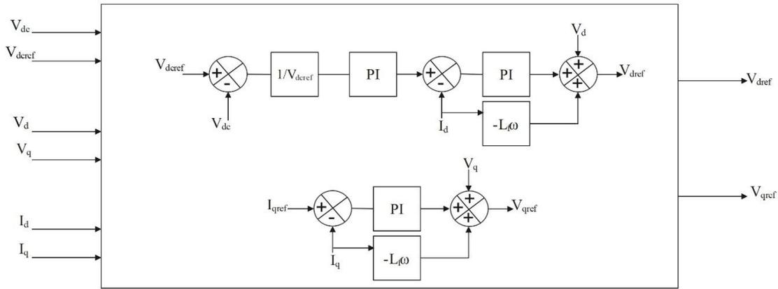
Figure 14 Control System for DC Voltage and dq Current Regulation for the Inverter NPC using PI controller
