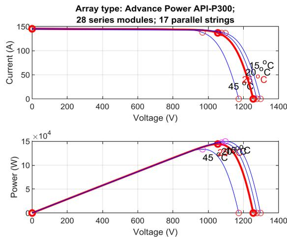
Figure 4 I-V and P-V Characteristics of Photovoltaic Array under Various Temperatures
