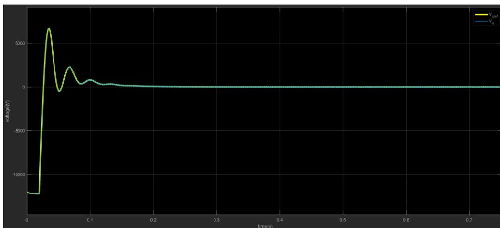
Figure 23 control of the output voltage in frame q  $V_q$  and  $V_{qref}$
