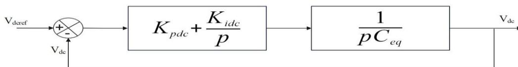
Figure 11 DC Voltage Regulation with PI Control Loop
