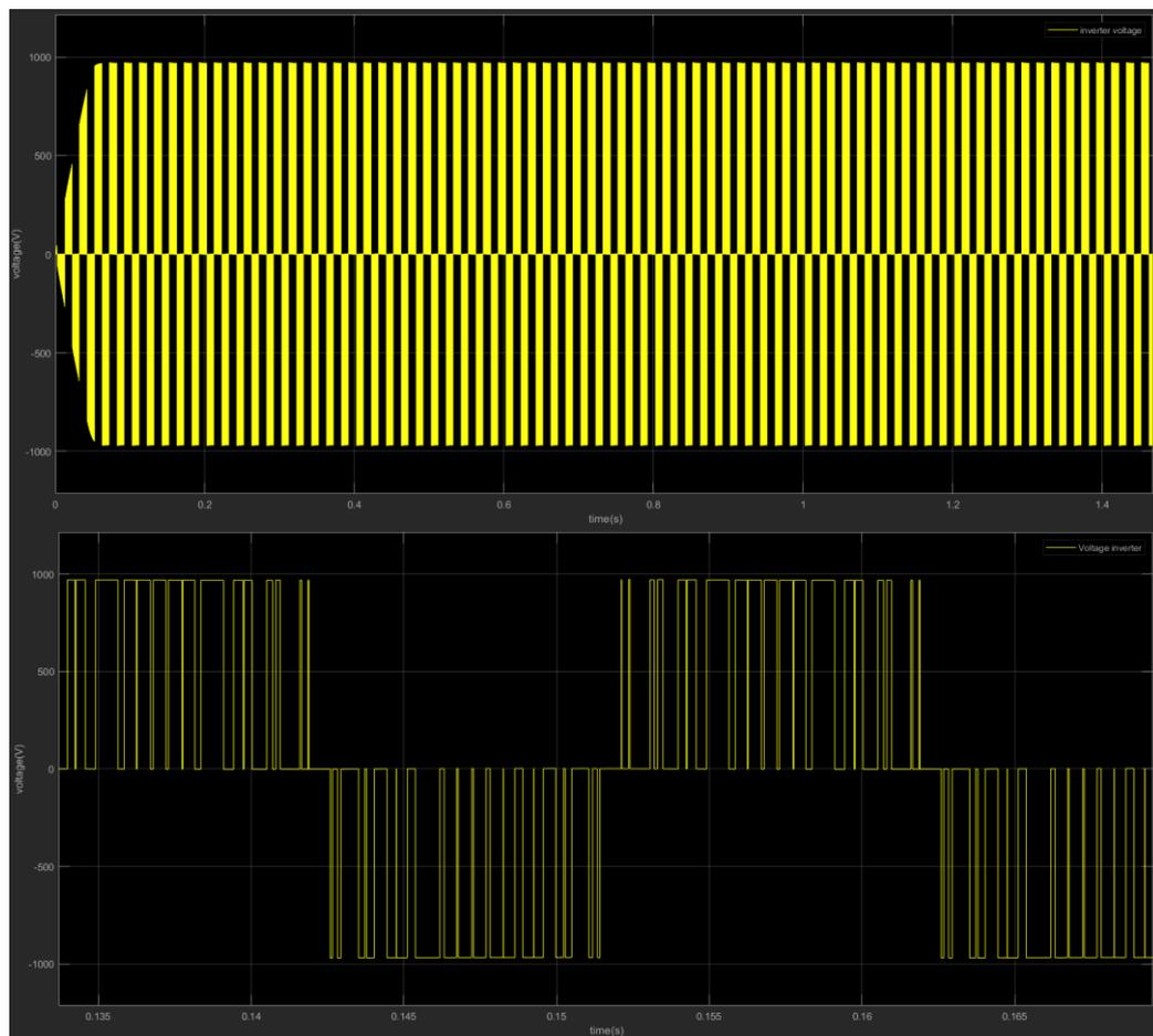
Figure 20 inverter voltage NPC 3level
