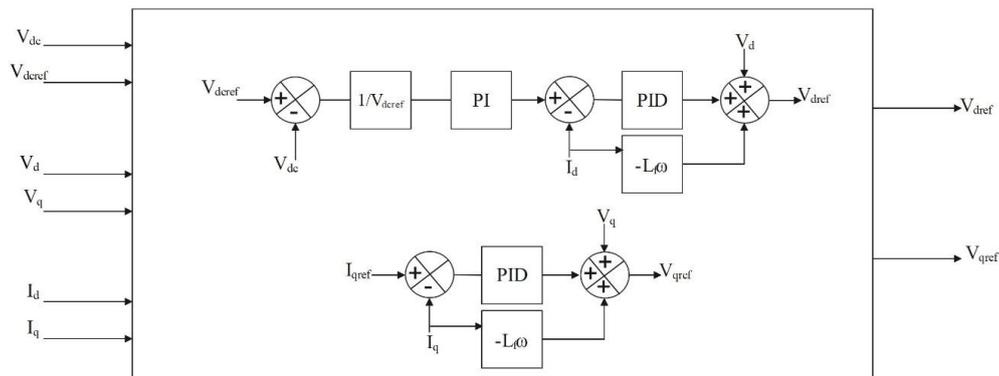
Figure 15 Control System for DC Voltage and dq Current Regulation for the Inverter NPC using PID controller
