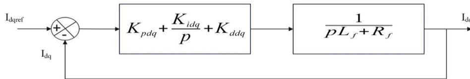
Figure 13 Current Regulation Using PID Control in dq Frame
