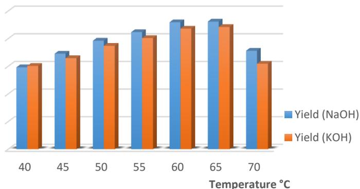
**Fig.2** Effect of reaction temperature (°C) on bone fat conversion
