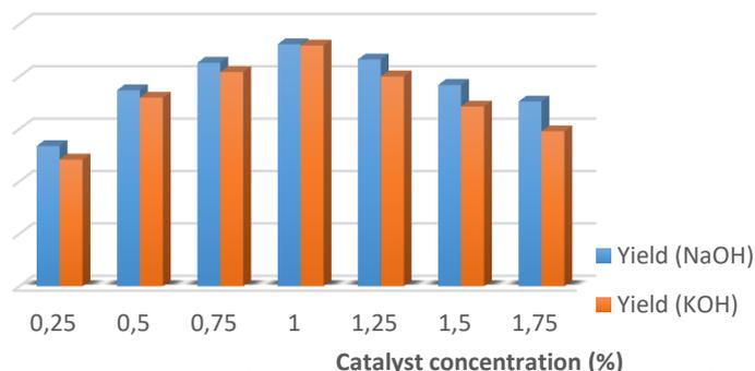
**Fig.1** Effect of alkali catalyst quantity on bone fat conversion
