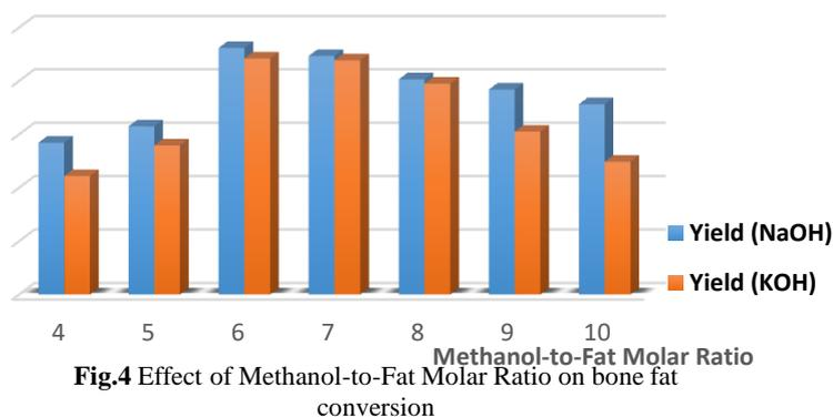
Fig.4 Effect of Methanol-to-Fat Molar Ratio on bone fat conversion
