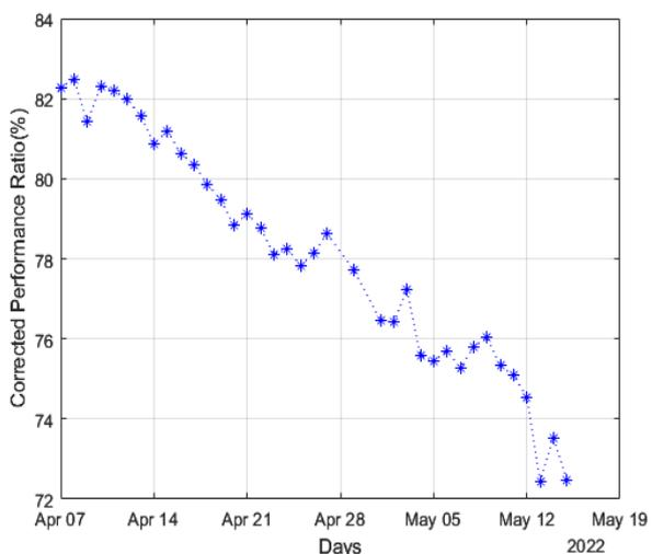
Fig. 7 Performance degradation due to dust
