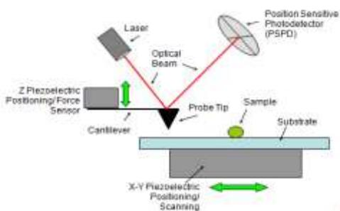
Fig.3 components of an AFM setup.
