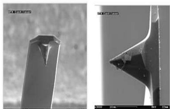
Fig.1 AFM Probe: Tip and cantilever of an AFM probe.
