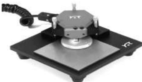
Fig.4 AFM scan head on the sample stage.
