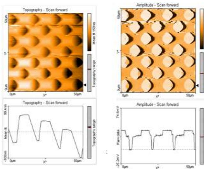
Fig.6: shows the topography and amplitude image of the microstructure sample at Vibration Amplitude Setting.
