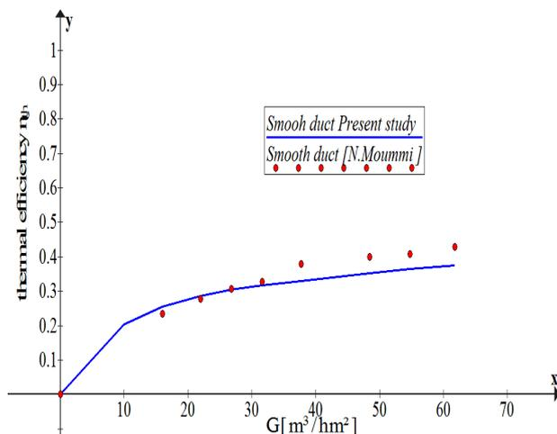
Figure 2: Validation of numerical results with experiments at constant flux of 900w/m<sup>2</sup>.
