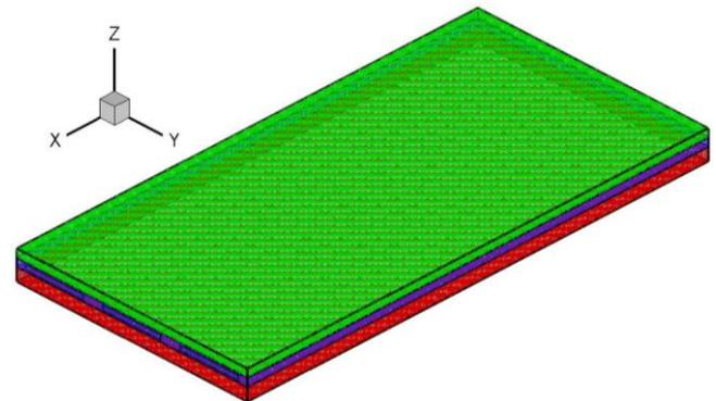
Figure 1: Mesh of the solar collector with Gambit 2.3.16
