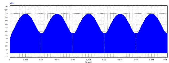
**Fig.4.Drain Source primary switch voltage**
