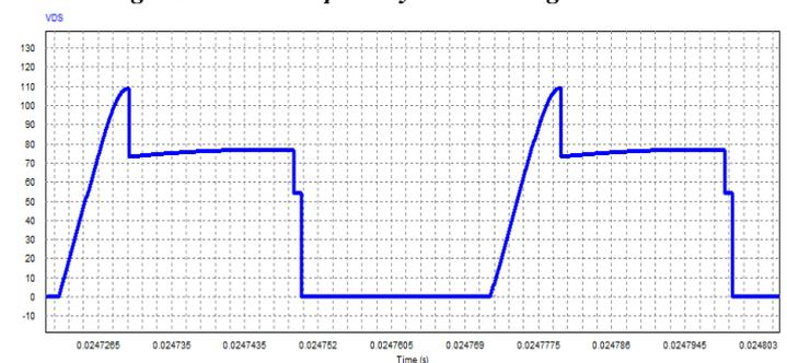
**Fig.5.Stress Drain Source voltage  $S_p$  switch**
