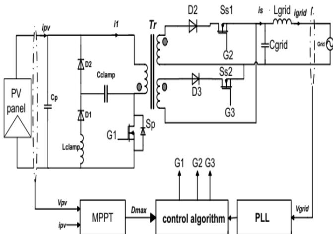
Fig.1. Flyback micro inverter and LCDD snubber
