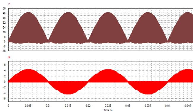
Fig.6. Primary current  $i_1$  and Secondary current  $i_s$
