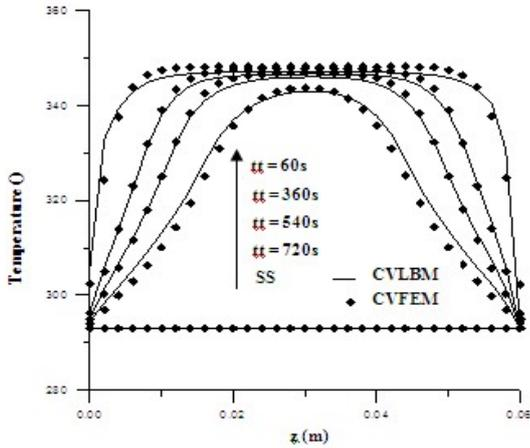
Fig. 4 Temporal Evolution of temperature along the axis of symmetry
