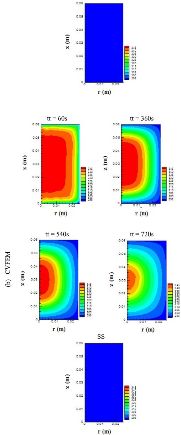
Fig. 5 Contours of the temperature at different times (a) CVLBM, (b) CVFEM
