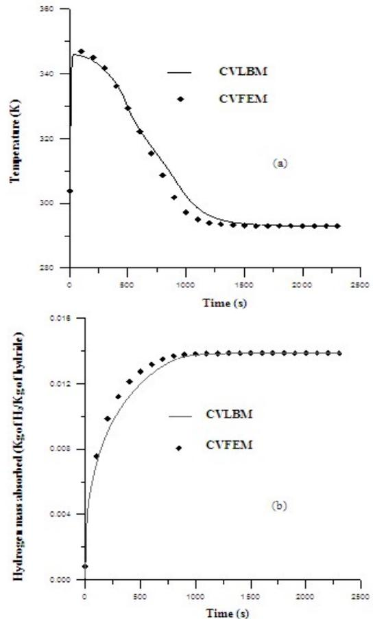
Fig. 3 Temporal evolution of (a) the hydride temperature and (b) the hydrogen mass absorbed
