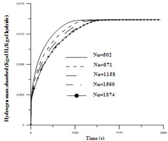
Fig. 2 Temporal evolution of the hydrogen mass absorbed for different number of nodes
