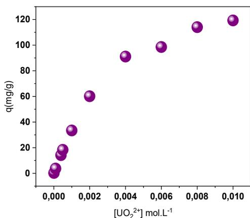
Fig.7 Sorption isotherm of Uranyl on organophosphorus resin as a function of initial metal concentration (V=5mL m=0.03g Θ= 300tpm).
