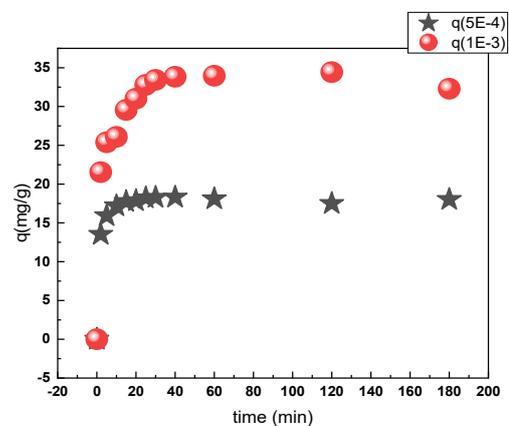
Fig.2 variation of the quantity absorbed of uranyl ions as a function of time
