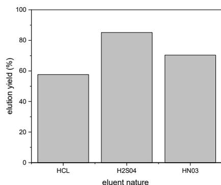
Fig.8 Effect of the nature of the eluent on the elution of Uranyl.
