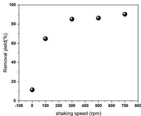
Fig.1 variation of the extraction yield according to the stirring rate.
