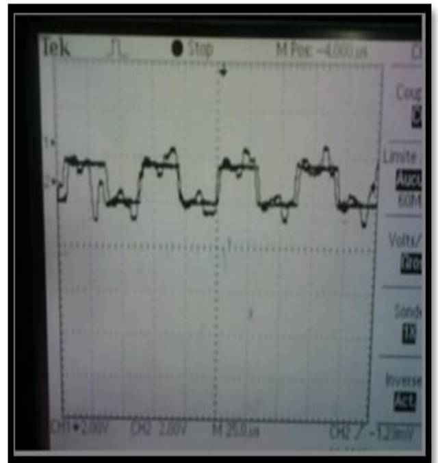
Fig. 7. Result of implementation of the oscilloscope set point and output signals "PID, system and DAC" design
