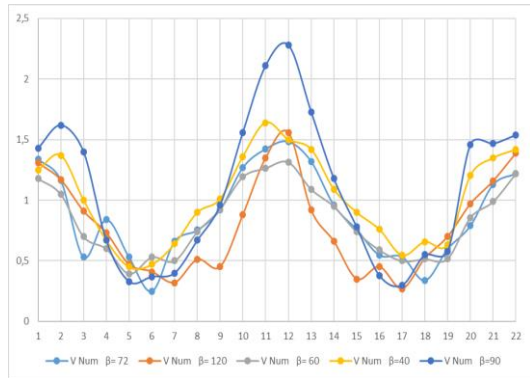
Fig 4. Speed profiles in tubes along the X-axis With V_e = 3.4 \text{ m/s} four several \beta angle
