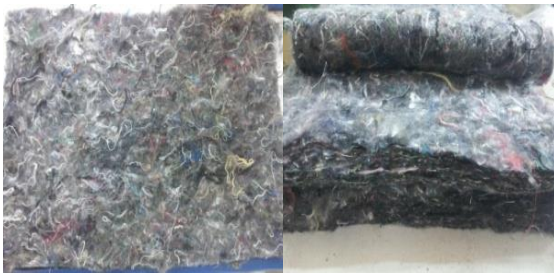
Fig 1 Non woven waste used as reinforcement
