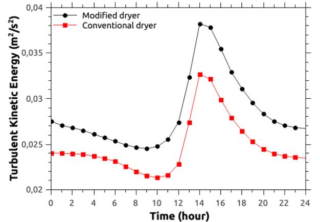
Fig. 3 Average turbulent kinetic energy intensity at 5 cm from drying rack
