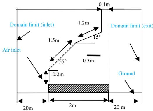
Fig. 1 solar dryer with the entrance at a 0.2 m height.
