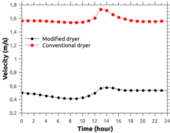
Fig. 4 Flow average speed at the inlet chimney section
