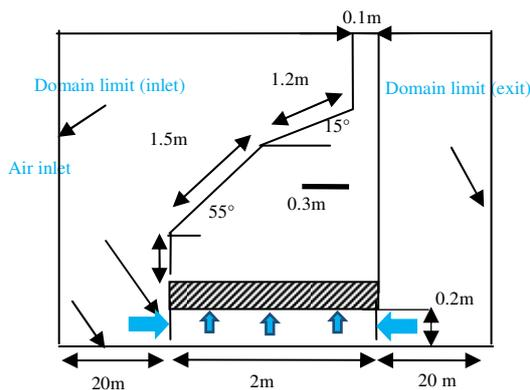
Fig. 2 solar dryer with the entrance at the bottom surface under the pebble bed.
