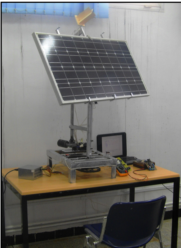
Fig.7 Solar tracker realized in the automatic laboratory
