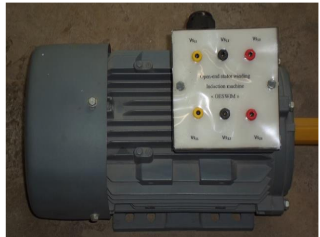
Fig. 6. Experimental prototyping of open-end winding induction machine
