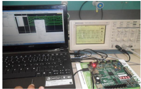
Fig.13 Photograph of the DSO display the control signals based on NR and generated from FPAG- XILINX
