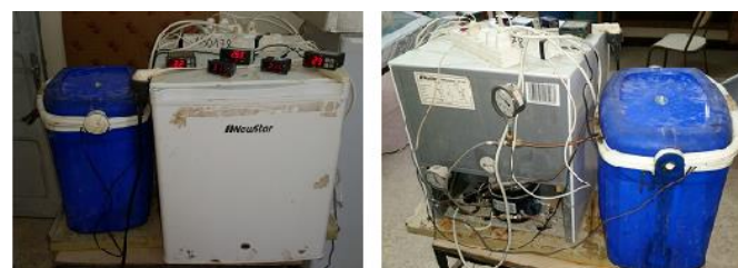
Fig.2: Domestic Refrigerator with Water Heater Tank photograph.
