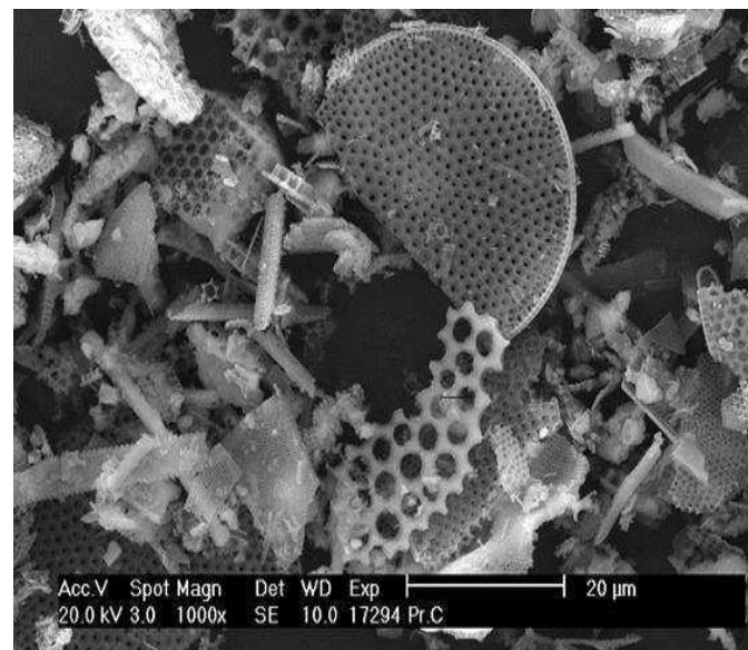
Fig. 3 SEM micrograph of the diatomite powder
