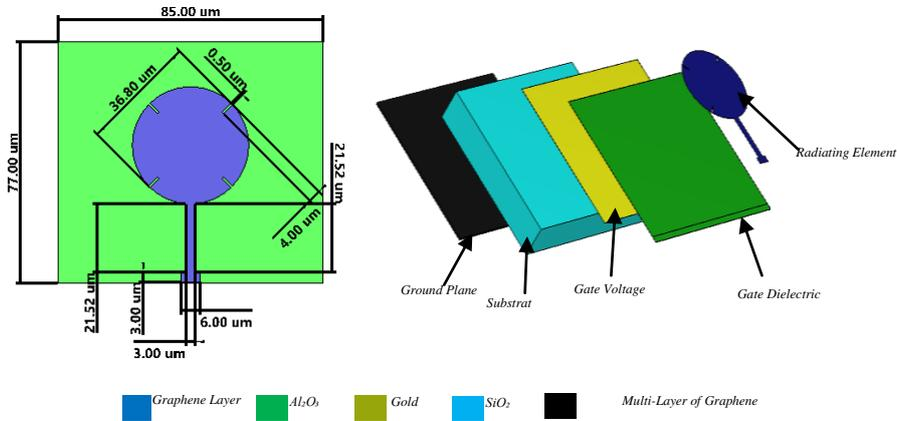
Fig. 2 Detailed geometry of the proposed nano-antenna.
