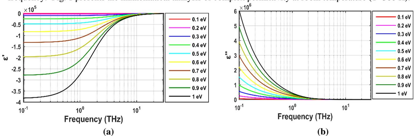
Fig. 1 Frequency-Dependent Graphene Permittivity for Various Chemical Potentials at 300 K: (a) Real Part and (b) Imaginary Part.
