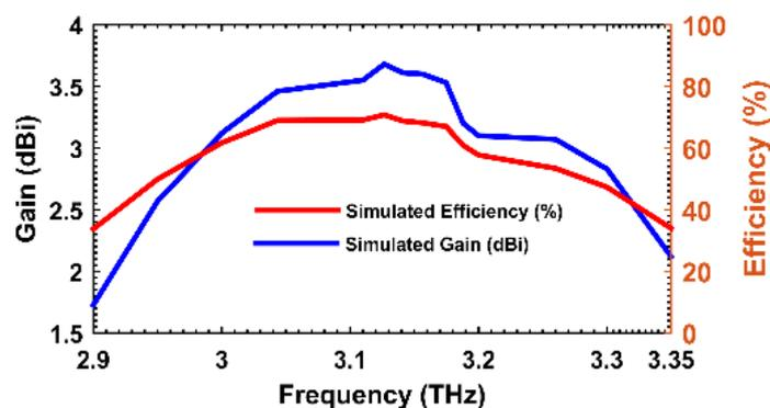
Fig. 5 Simulated gain and radiation efficiency of the proposed nano-antenna across the tunable frequency range.
