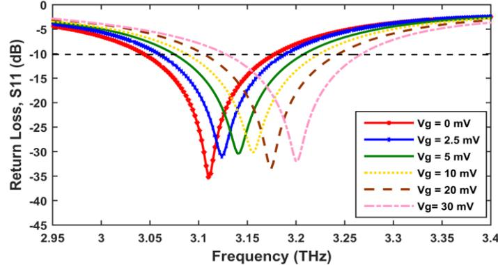
Fig. 3 Return loss simulations of the proposed graphene nano-antenna under different gate voltages.
