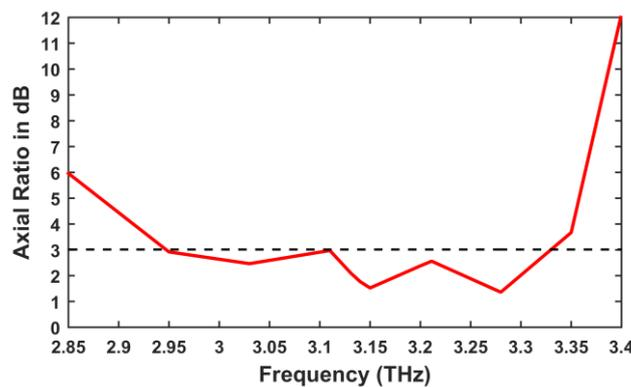
Fig. 4 Axial ratio performance of the proposed nano-antenna across the operational frequency range.
