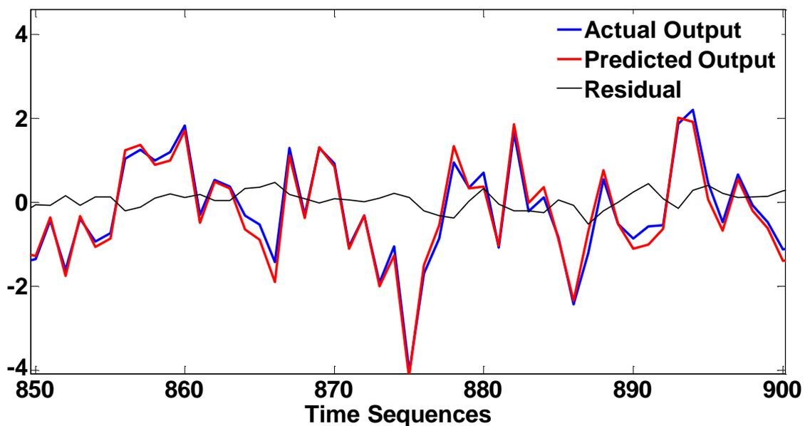
Fig. 3. Residual of SISO system using RGELS algorithm between  $n = 850$  and  $n = 900$ .
