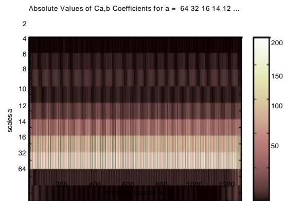
Fig. 12 Scalogram of CWT of the system degraded motor - reducer following an unbalance
