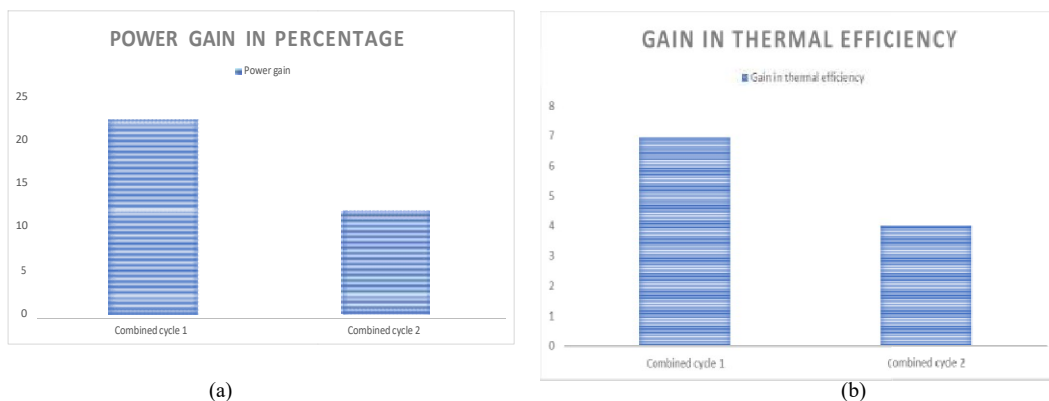
Fig.6 Comparison of the gain in performances obtained with the two combined cycles (a): useful power; (b) : thermal efficiency
