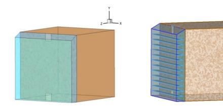
Fig.1:3D Model of the Transparent Trombe Wall
