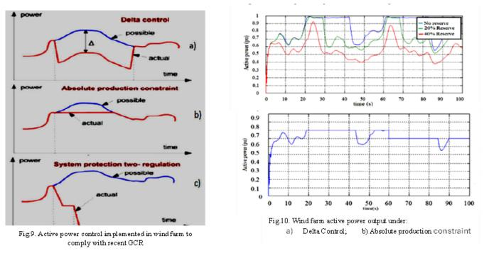
These controls have been tested to operate the wind power plant with power reserve or with curtailment (Fig.10). Similarly, the emergency shutdown of the wind power plant was tested, following the instruction of the network operator, while respecting the ramp-down rates required by the Grid Code.
