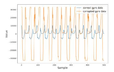
Figure 6:Corrupted vs. correct gyroscope values
