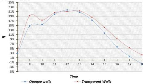
Fig.3: Thermal Efficiency of Transparent Trombe Wall unit with transparent and opaque's lateral walls and roof for a winter solstice day
