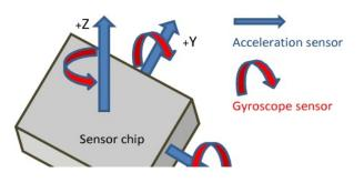
Figure 4:IMUs axis and orientation
