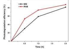
Fig.6 Photodegradation efficiency of MG and RhB for different sun light irradiation time for T45S45 sample.
