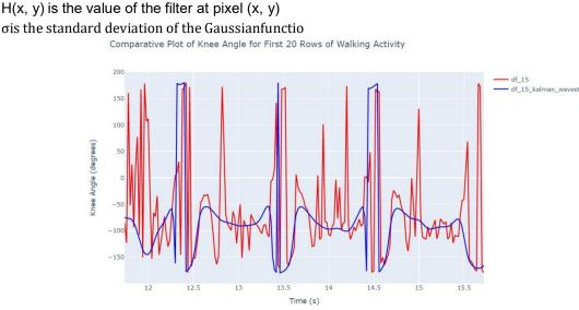
Figure 9: Original vs denoised data usingGaussianfilter
