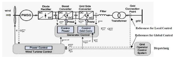
Fig.8. GFM control in Wind plant: Local control according to PoC references; Centralized control from the dispatching
