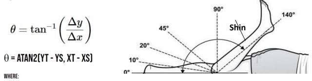
Figure 3:Knee angle estimation based on acceleration of the shin and thigh
