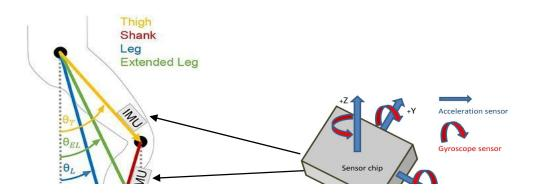
Figure 5: Gyroscope and accelerometer placements
