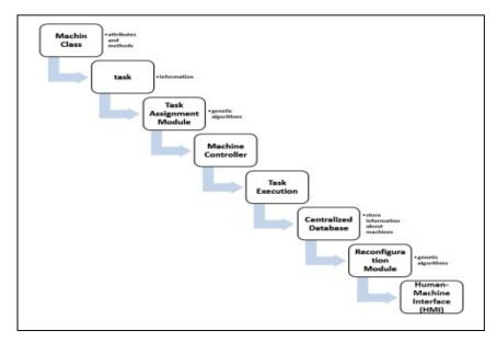
Fig. 1 A proposed architecture for intelligent manufacturing systems.
