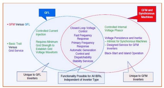
Fig.2-features and grid services of GFL IBRs , GFM IBRs and Synchronous Machines [3]
