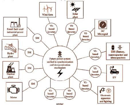
Fig.1- The application of conventional Synchronous Machines (SM) and Voltage/Current (VI) Based Inverter
