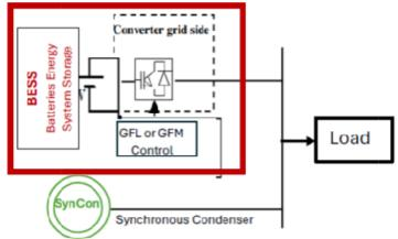
Fig. 15. Microgrid configuration: BESS (2.2MW) under GFL or GFM control with or without SynCon (2.5 MVA) [15]
