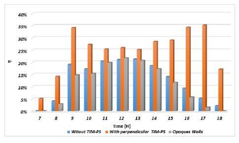
Fig.4: Thermal Efficiency for TIM-PS and Conventional Transparent Trombe Wall
