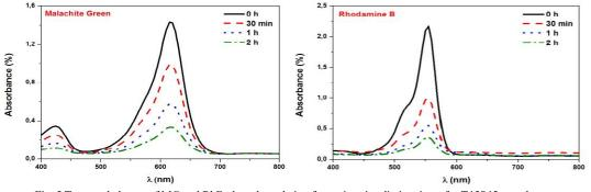
Fig. 5 Temporal change of MG and RhB photodegradation for various irradiation times for T45S45 sample.
