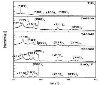
Fig. 1 XRD Spectra of chemically sprayed TiO<sub>2</sub>-SnO<sub>2</sub>:F thin films deposited at different oxides' contribution.
