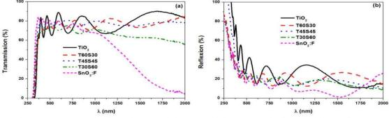
Fig.2 Transmission (a) and Reflexion (b) spectra of TiO2-SnO2:F thin layers deposited at different oxides' contribution.
