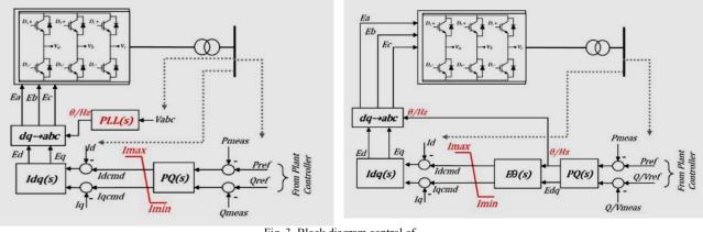
Fig. 3. Block diagram control of a) GFL inverter b) GFM inverter
