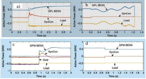
Fig.16- MicroGrid operation on islanded mode [15] a)GFL control with SynContripping c)GFM control with SynCon: d) GFM control
