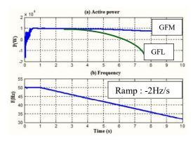
Fig.7. PV Frequency Ride through with GFM/GFL Control
