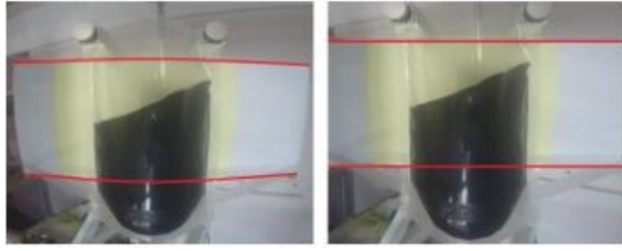
Fig. 5. Original image (left) and undistorted image (right). Note the shape red lines corresponding to top and bottom edges of the back white screen, before and after the undistortion
