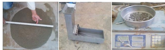
Fig. 3 Qualification test of self-compacting concrete: a-Slump flow, b- L-Box and c-Stability in sieve
