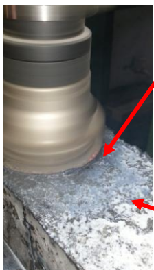
Figure 6: appearance of a flame Figure 7: disappearance of the flame until has speed 630 and 315tr/min speed 160tr/min.
