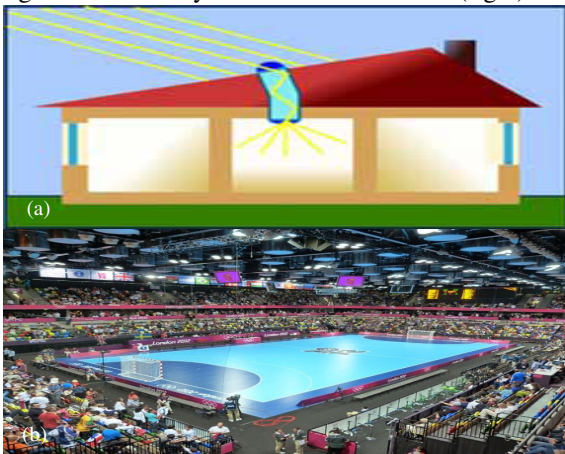
Fig. 8. a- Light tubes. b-The Copper Box, venue for Handball at the 2012 Summer Olympics, makes use of light tubes to reduce energy use.
