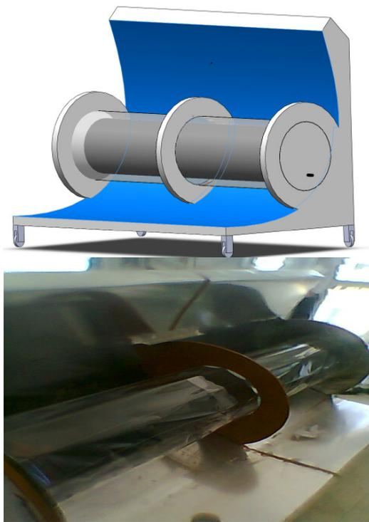
Fig.6. Chauffe-eau solaire cylindro-parabolique CESC
