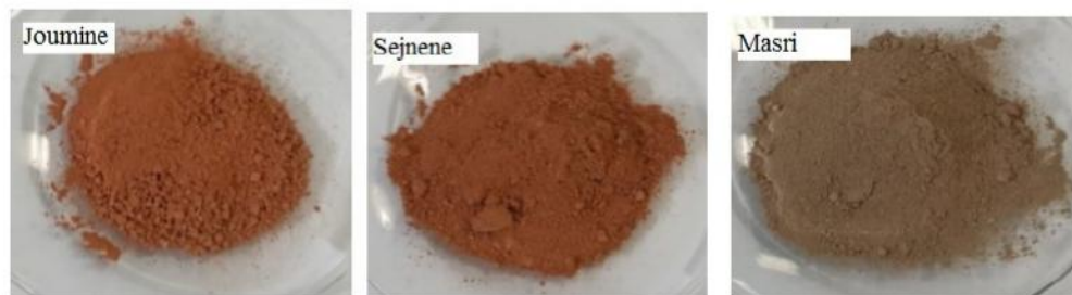
Fig. 3 visual appearance of sediments after grinding
