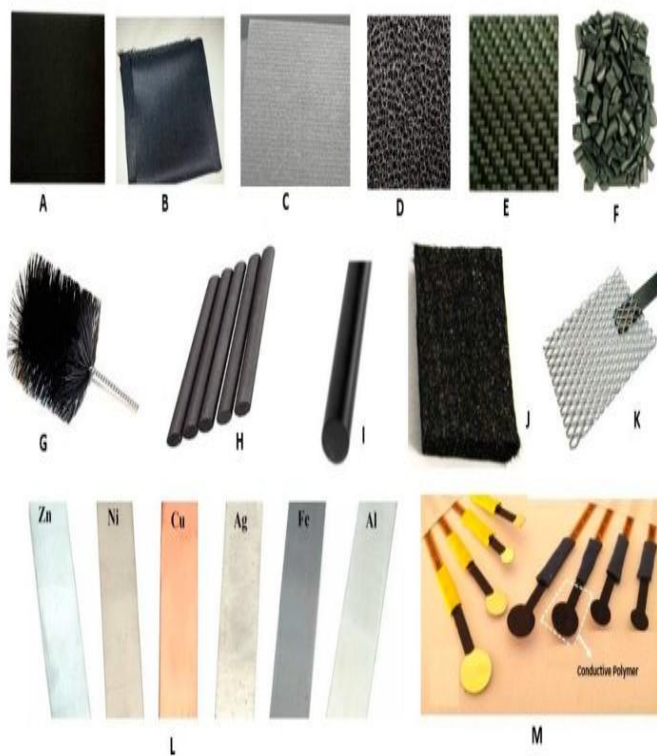
Fig.6 Mostly used anode electrodes (A) carbon paper, (B) carbon cloth, (C) carbon fibre, (D) reticulated vitrified carbon, (E) carbon mesh, (F) graphitic granular, (G) carbon brushes, (H) graphite rod, (I) polycrystalline graphite, (J) carbon felt, (K) platinum mesh, (L) different metal electrode strips, (M) conductive polymer-based strips..[25]
