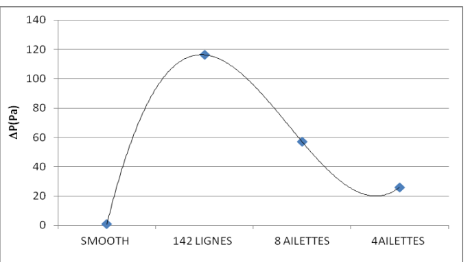
Fig.9: Variations of pressure drop at different fins Numbers for G=40[m 3 /hm 2 ].
