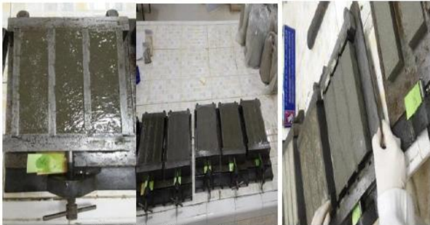
Fig. 1 Manufacture of mortar specimens
