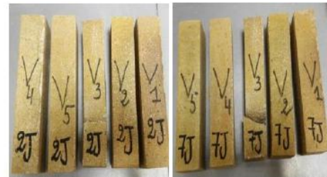
Fig. 5 Test specimens after heat treatment at 1400°C.
