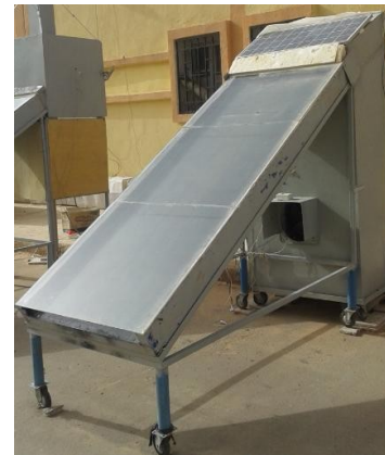
Fig. 2 Photo of the indirect solar dryer.
