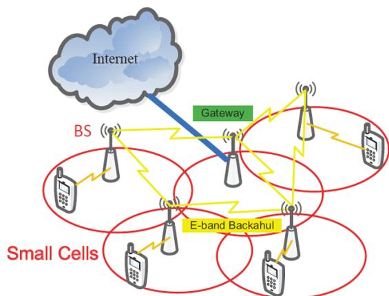
Fig. 3. E-band backhaul for small cells densely deployed [9].
