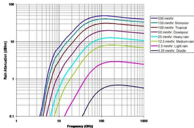
Fig. 6. Rain attenuation at microwave and mm-Wave frequencies.
