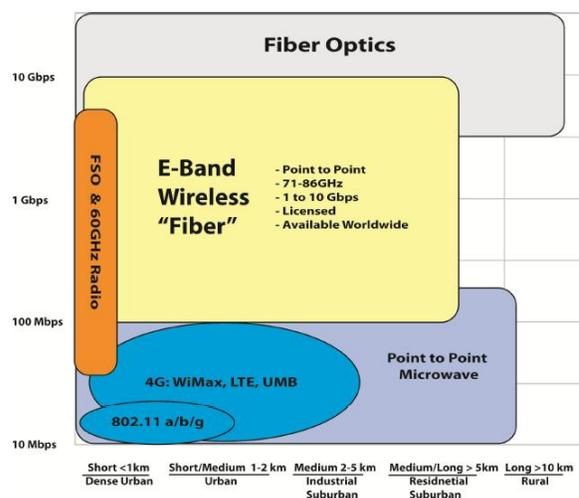
Fig. 1. The major higher capacity wireless technologies.
