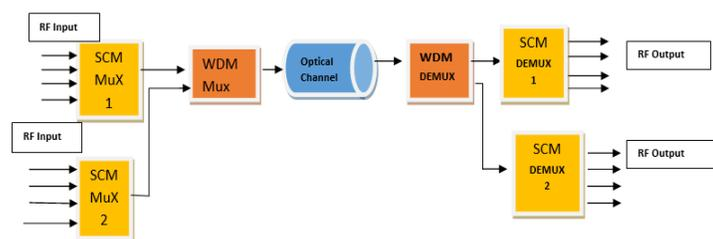
Figure.5. the architecture of SCM/WDM
