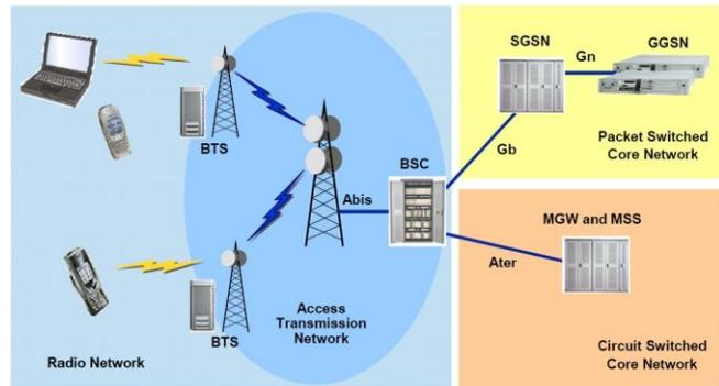
Figure.3. the classical architecture of mobile network system
