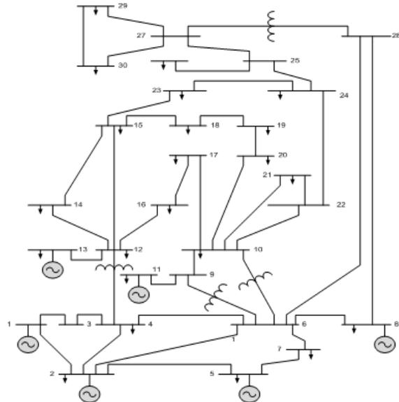
Fig. 2 Single line diagram of IEEE-30bus [2]
