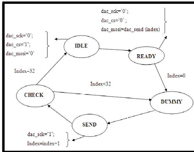
Fig. 7. State diagram of the VHDL program DAC
