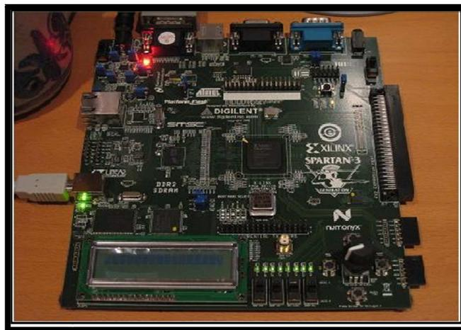
**Fig. 10.** Circuit Xilinx XC3S700A Spartan 3A Starter Kit
