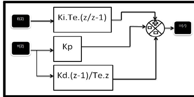
**Fig. 1.** A block diagram of PID controller
