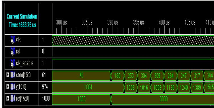
**Fig. 5.** Simulation of PID control system by the ISE simulator
