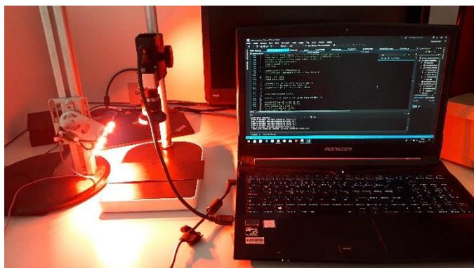
Fig. 6 Investigation of Effect of Exposure Time and Light Angle On Image Quality
