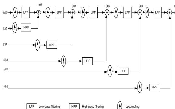
Fig. 4 The Inverse DWT filtering process
