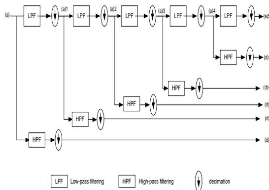
Fig. 3 filtering Process
