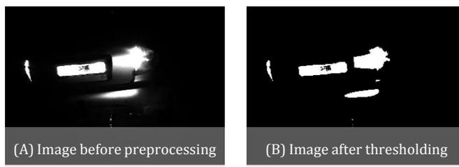
Fig. 4 Binary Thresholding of IR Image.
