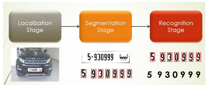
Fig. 1 The main stages of a typical LPR system
