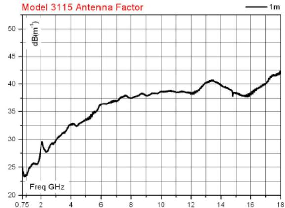
Figure 2. Model 3115 Typical Antenna Factor
