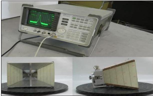
Figure 1. Double-ridged waveguide horn antenna with spectrum analyzer
