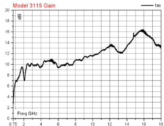
Figure 3. Model 3115 Typical Antenna Gain
