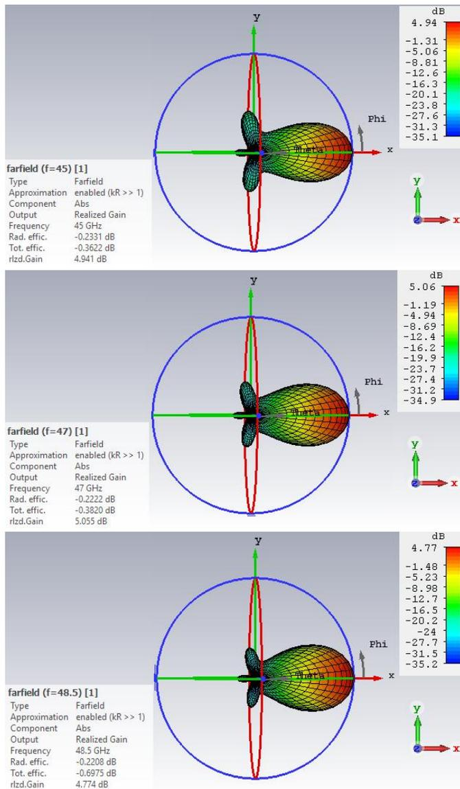
Fig.8: The realized gain for three different frequencies
