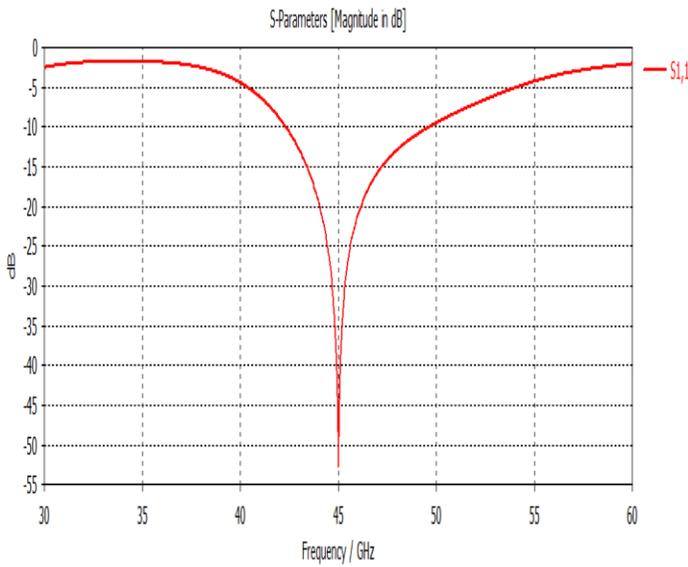
Fig.6: Return loss (S11) and steady state parameters.
