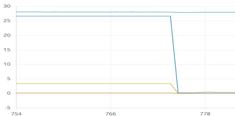
Fig. 29. Curve Displayed on Arduino Serial Plotter for Total Shading
