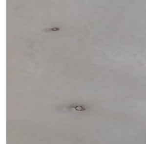
Fig. 12 Perforations in the PE solid barrier caused by electrical breakdown
