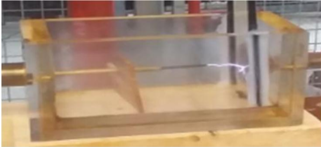
Fig. 11 Formation of the electric arc in air with solid barrier
