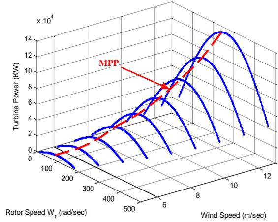
Fig. 3 Turbine power versus rotor speeds and wind speed
