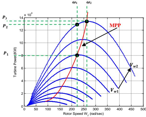
Fig. 4 Turbine power versus rotor speeds of generator
