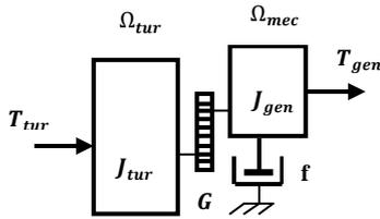
Fig. 2 Mechanical model simplified of wind turbine
