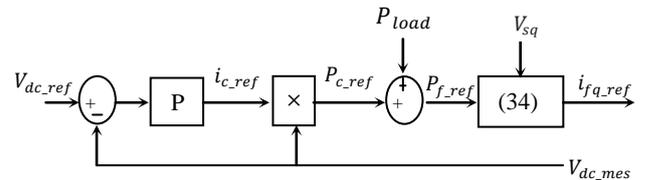
Fig. 9 Bloc diagram of DC bus control.
