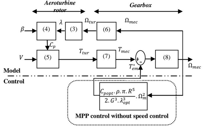
Fig. 6 Block diagram without speed control
