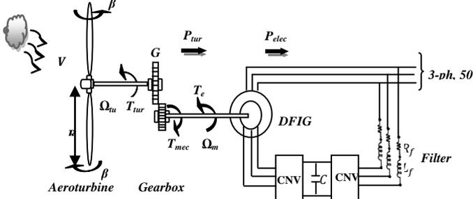
Fig. 1 Schematic diagram of DFIG wind turbine
